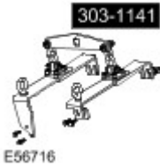
Engine lifting Cradle 303-1141
